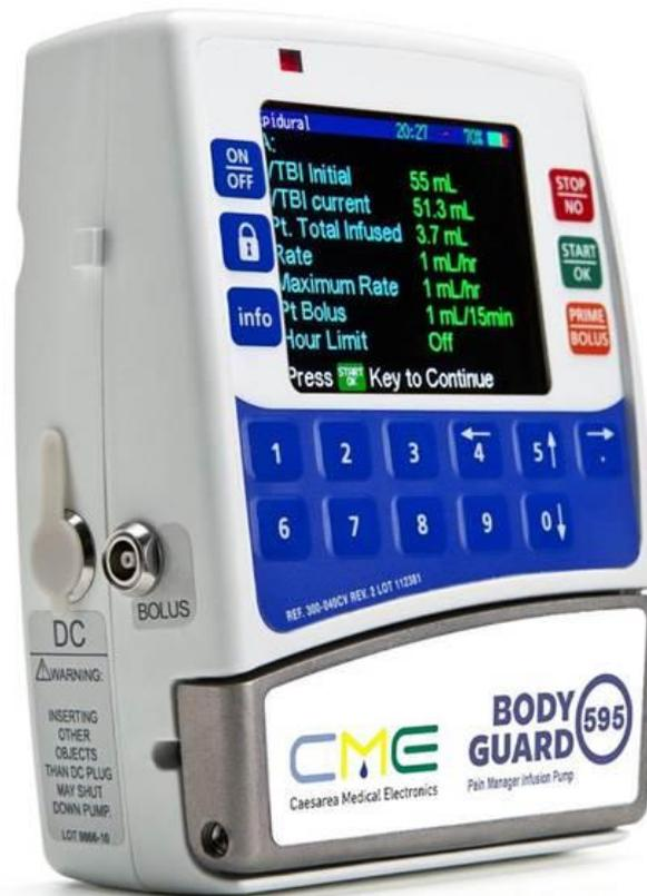
The Bodyguard 595™ delivers a continuous infusion. It also allows patient-controlled intermittent bolus doses to be given as needed using the bolus cord. This has a lock-out facility to limit frequency of dosing. The prescribed medication is formulated in pharmacy and dispensed in a sterile bag of saline (100mL, 200mL or 500mL).
